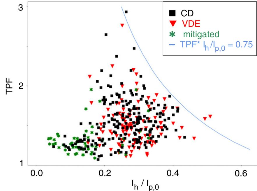
Pautasso et al. (AUG) have extensive measurements of the halo currents and observe significant variation associated with the type of disruptions and mitigation.
