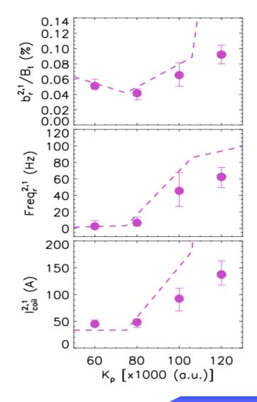
Good comparison between experiment (dots) and RFXlocking (traces) for m=2, n=1 control in 2<q(a)<2.5 RFX-mod tokamak shots
