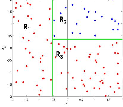
the algorithm selects a splitting value to partition the dataset, by **minimizing** an **impurity** measure:
