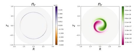
The eigenfunction of the tearing mode (left) at  $S = 10^4$  is localized near the q = 2 rational surface with poloidal mode number m = 2. The fastest growing mode at  $S = 10^2$ , has m = 1, and is not localized near the rational surface.
