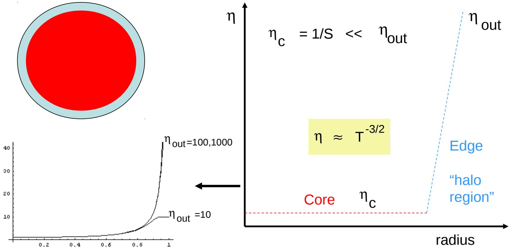
Apart the arbitrariness of  $\eta_{out}$  the halo region is self-consistently determined by the time evolution of temperature
