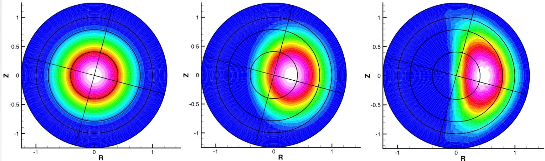
Contours of constant pressure at  $t=0$ ,  $3 \tau_A$  from maximum displacement, and  $1 \tau_A$  from maximum displacement.
