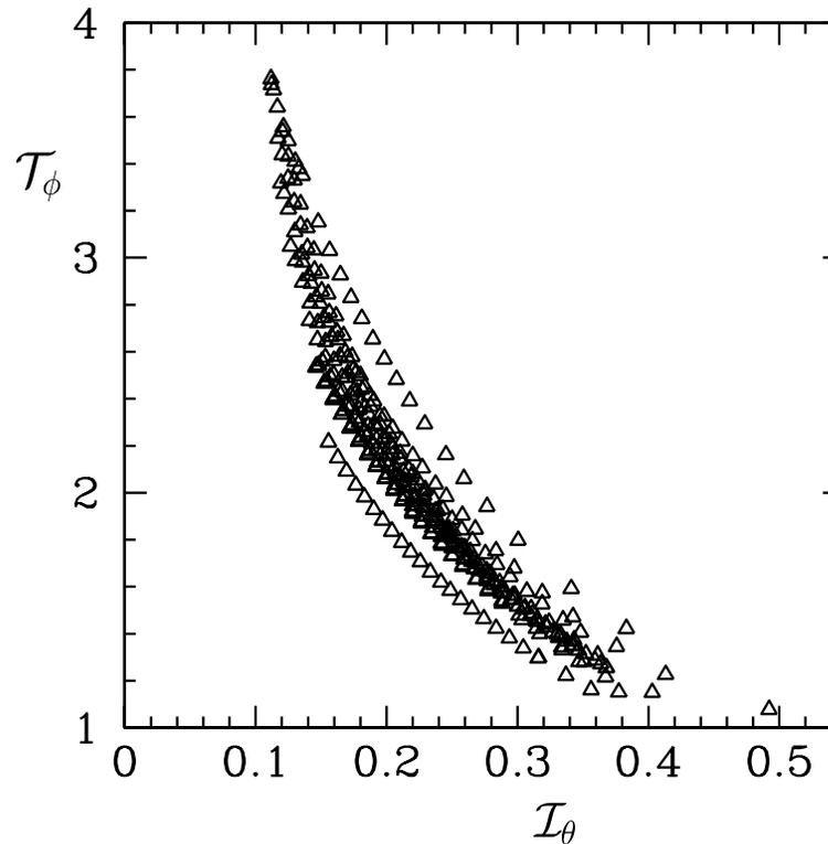
Ansatz that current quench triggered when halo current fraction exceeds critical value reproduces inverse relation between TPF and poloidal halo current fraction seen experimentally.
