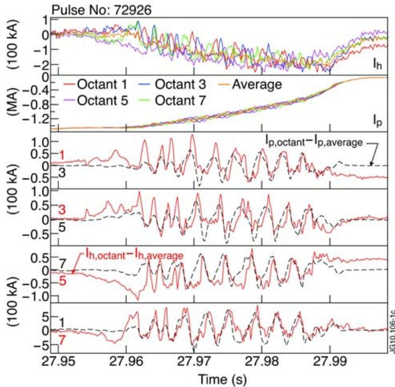
The asymmetric component of the poloidal halo current and the asymmetric component of the toroidal plasma current shifted toroidally by  $\pi/2$  (Riccardo, 2010)
