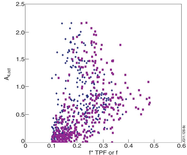
Time integrated measure of the  $I_p$  asymmetry ( $A_{4oct}$ ), shows the maximum sideways impulse force is not coincident with either maximum spatially averaged halo fraction ( $f$ ) or with the maximum local halo fraction ( $f^* \text{ TPF}$ ) (Hender)
