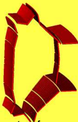
One toroidal sector of copper stabilizers (8728 triangles)
