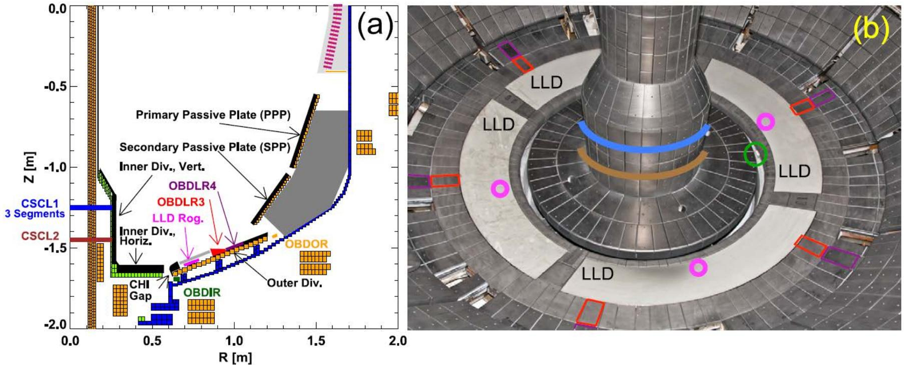
Halo current is inferred from transient TF measurements under several divertor tiles and plates at about six toroidal locations. Transient vessel forces are not measured.
