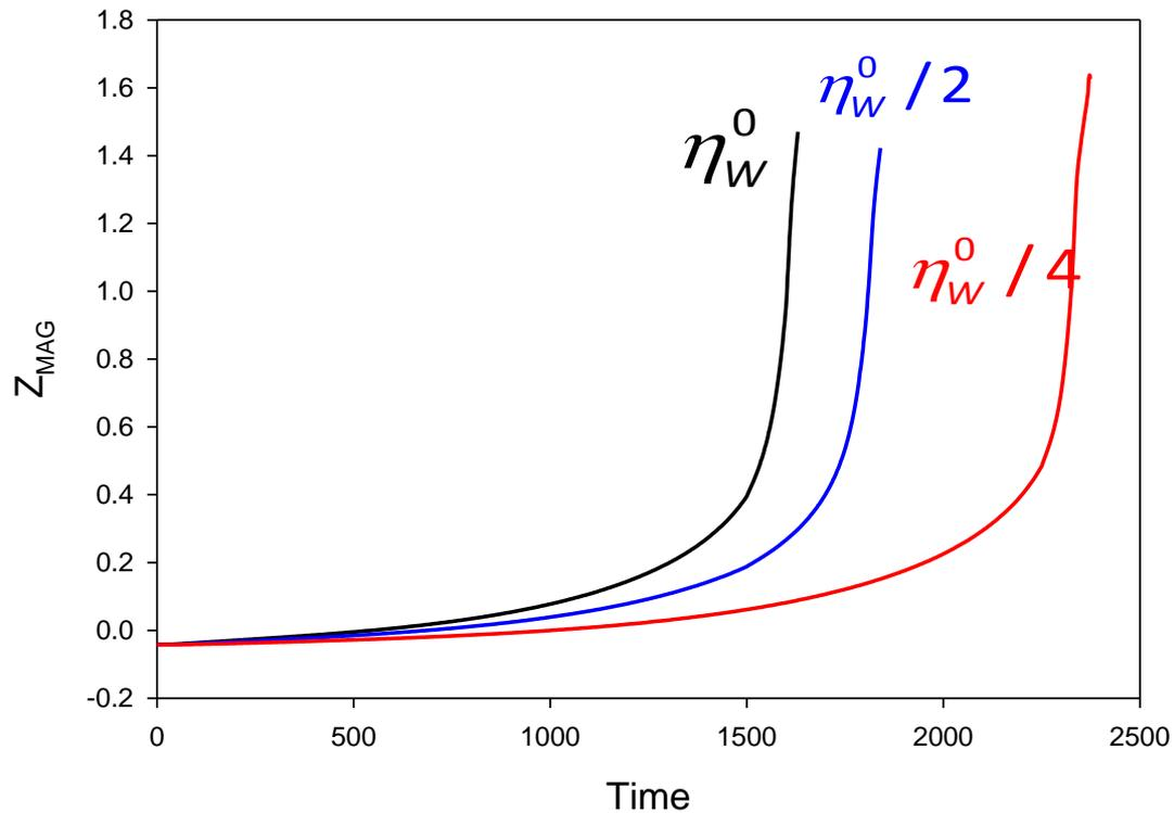
Growth rate scales inversely with wall resistivity  $\eta_w$  as expected
