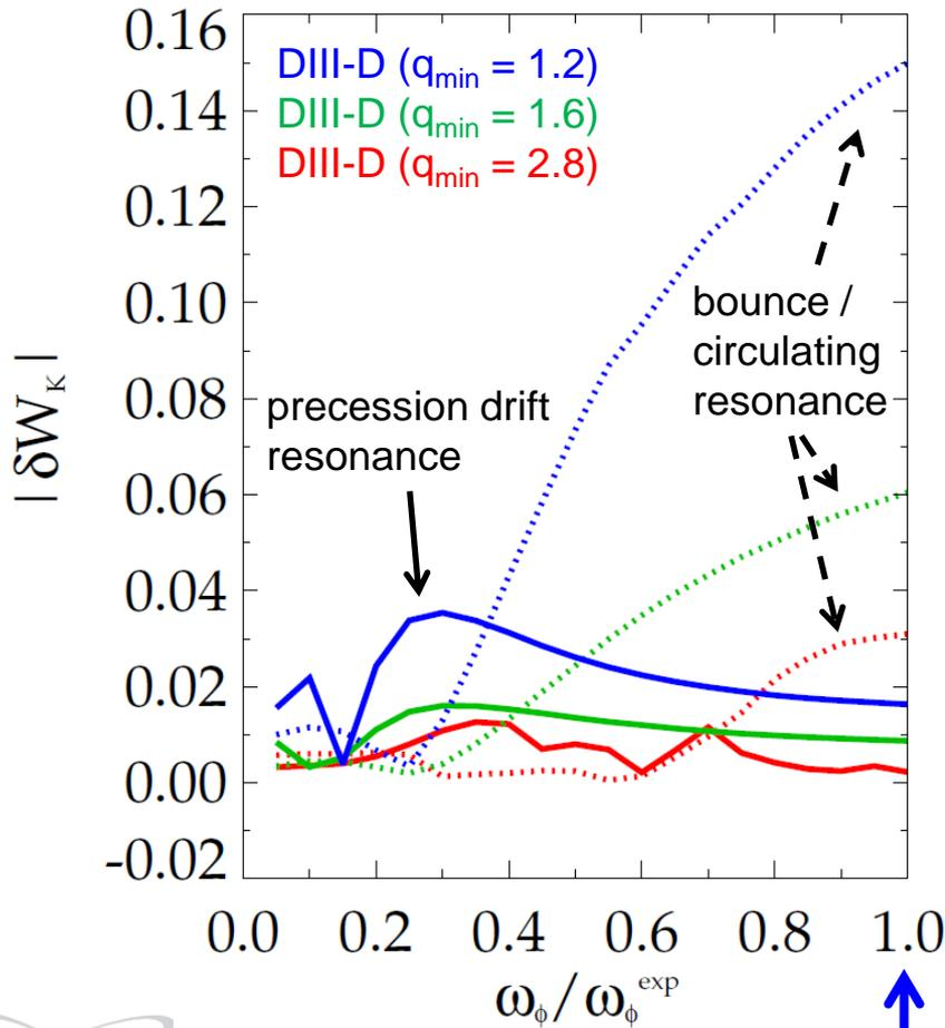
Measured plasma response to 20 Hz,  $n = 1$  field vs  $q_{\min}$
