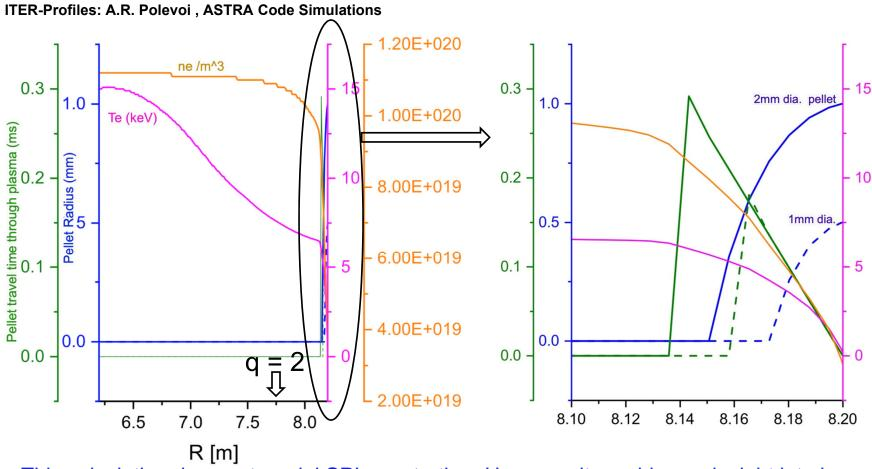
This calculation does not model SPI penetration. However, it provides an insight into how deep a single pellet could be expected to penetrate in high energy ITER plasmas.
