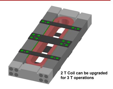
**Coil Supports Designed to Restrain Coil Motion**
