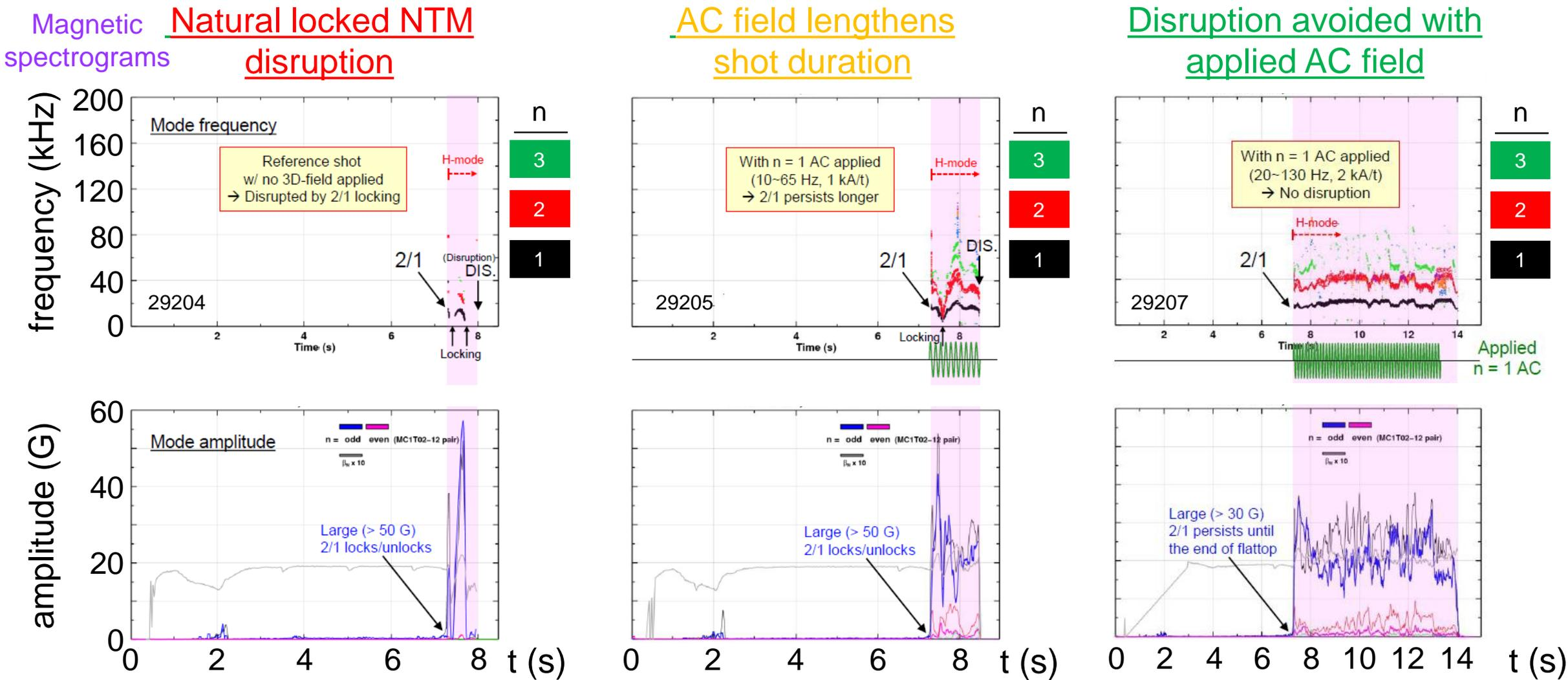
NOTE: applied AC field frequency is  $\ll$  mode rotation (due to boundary value field alteration? analysis continues)
